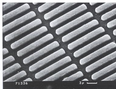
Fig. 3. LGC Promochem 12  $\mu\text{m}$  long shape standards attached to a silicon substrate. From Kelly and Kazanjian, 2005.
