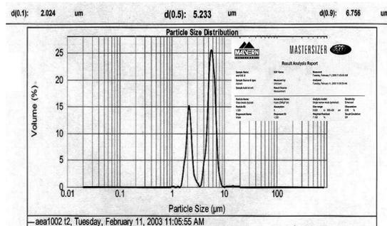
Fig. 1. Bimodal distribution corresponds to diffraction along both the minor and major chords. This response was noted regardless of the flow speed or the laser diffraction system used (Beckman-Coulter, Horiba, Malvern, and Sympatec). From Kelly, 2004.
