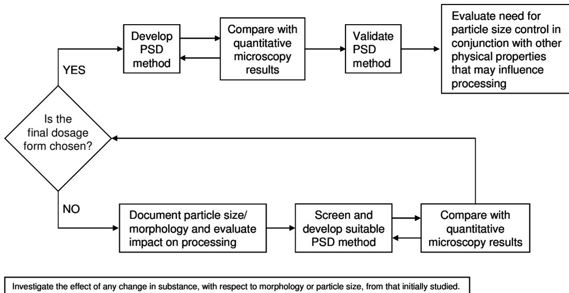
Fig. 4. The proper way of selecting and validating a particle-sizing method. From Kelly (2004).
