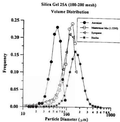
Fig. 2. An example of a discrepancy between laser diffraction analysis (using either Mie or Fraunhofer optical model) and time-of-flight technique (corroborated by image analysis). From Etzler and Deanne, 1997.
